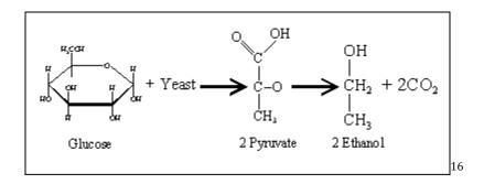
The yeast converts the 3-carbon pyruvate chains into ethanol by removing a carbon dioxide molecule from the pyruvate using the enzyme pyruvate decarboxylase, creating acetaldehyde, and then converting the acetaldehyde into ethanol using the enzyme alcohol dehydrogenase.<sup>17</sup> The diagram above briefly illustrates the chemical conversion of glucose to ethanol.
